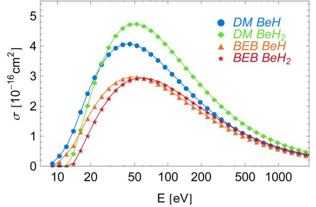
**Fig. 3.** (Color online) Electron-impact ionization cross section of BeH and BeH<sub>2</sub> from the DM and BEB methods.
