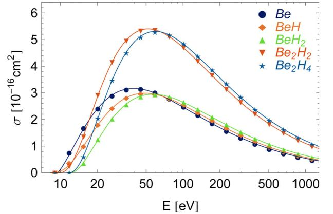
**Fig. 7.** (Color online) Cross sections (solid lines) obtained from fitting the BEB values (symbols) to equation (3).
