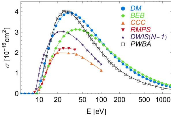
**Fig. 1.** (Color online) Electron impact ionization cross section of Be: Deutsch-Märk (DM) cross section (circle), binary-encounter-Bethe (BEB) (diamond), CCC (triangle) [20], RMPS (inverted triangle) [20], DWIS(N-1) (star) [23] and PWBA (square) [24,25] calculations.
