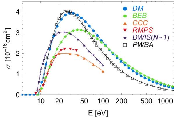
**Fig. 1.** (Color online) Electron impact ionization cross section of Be: Deutsch-Märk (DM) cross section (circle), binary-encounter-Bethe (BEB) (diamond), CCC (triangle) [20], RMPS (inverted triangle) [20], DWIS(N-1) (star) [23] and PWBA (square) [24,25] calculations.
