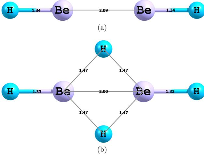
**Fig. 4.** (Color online) Minimum-energy structures of (a) Be<sub>2</sub>H<sub>2</sub> and (b) Be<sub>2</sub>H<sub>4</sub> from QCISD/aug-cc-pVTZ calculations.
