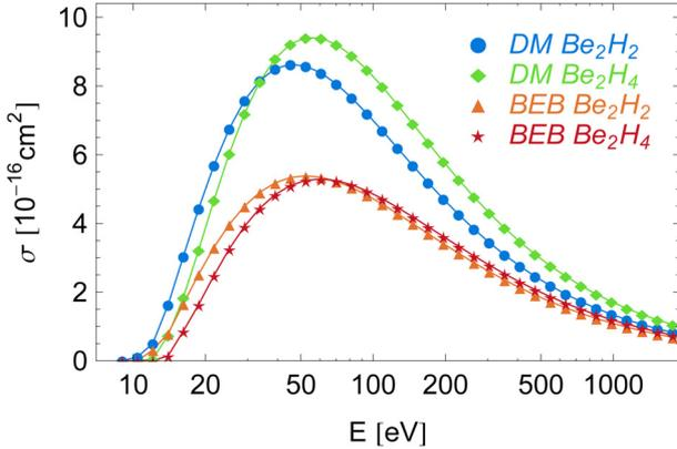
**Fig. 5.** (Color online) Electron-impact ionization cross sections of Be<sub>2</sub>H<sub>2</sub> and Be<sub>2</sub>H<sub>4</sub> from the DM and BEB methods.
