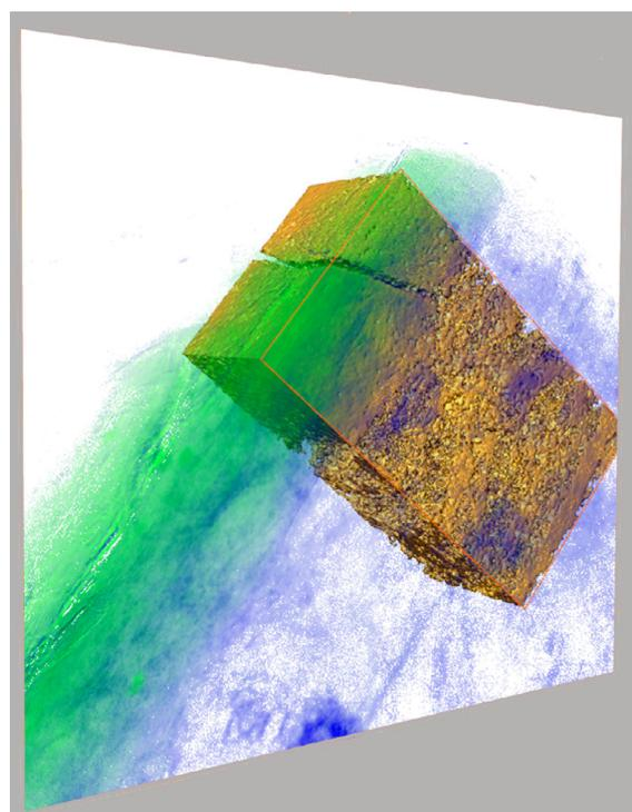
**Fig. 7.** 3D tomographic data obtained at SSRL (Stanford, USA) with the 2D mosaic phase map of the campanian pottery [67].
