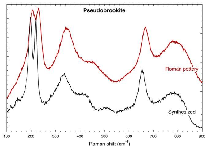
**Fig. 5.** Comparison of Raman spectra measured on synthesized pseudobrookite and marbled terra sigillata (Roman pottery) containing pseudobrookite crystals (Tian Wang, CEMES, private communication).
