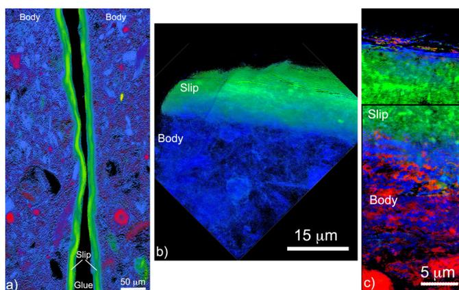
**Fig. 6.** Phase maps deduced from Full-field XANES analysis performed at (a) ESRF (Grenoble, France) for a campanian, and at SSRL (Stanford, USA) (b) for the same campanian and (c) for a presigillata [67].
