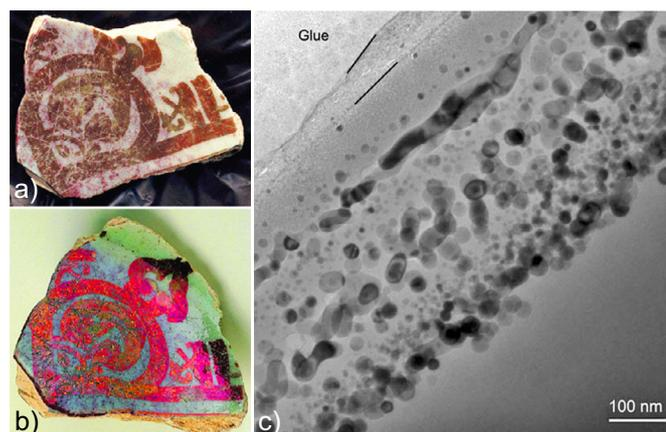
**Fig. 2.** (a, b) Lustre ware from Fatimid period, 12th century. AD where the colour change from brown (scattering light) to pink (specular position) and (c) TEM image of silver nanoparticle distribution responsible of the shiny aspect of this kind of lustre [37].
