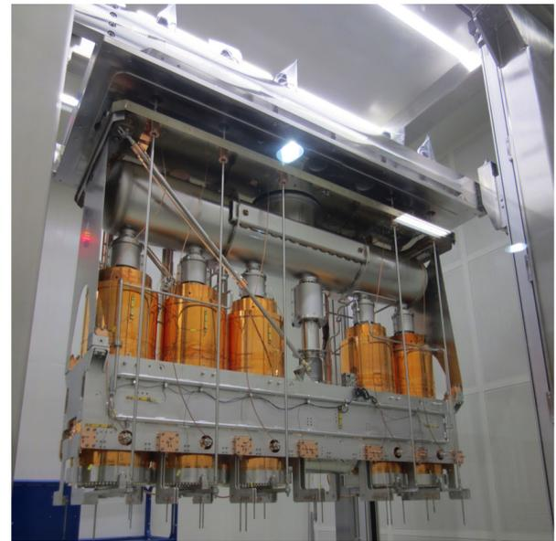
**Fig. 7.** The picture, taken in April 2015, shows the complete assembly of the first cryomodule. One can see the 5 cavities, the helium vessel on the top and the support frame hiding the solenoid placed between the third and fourth cavity.
