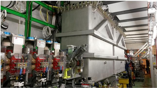
**Fig. 9.** The ISOLDE post-accelerator with two cryomodules is shown in the photo taken inside the linac tunnel. Radioactive beams up to 5.5 MeV/u are expected for the end of August 2016.
