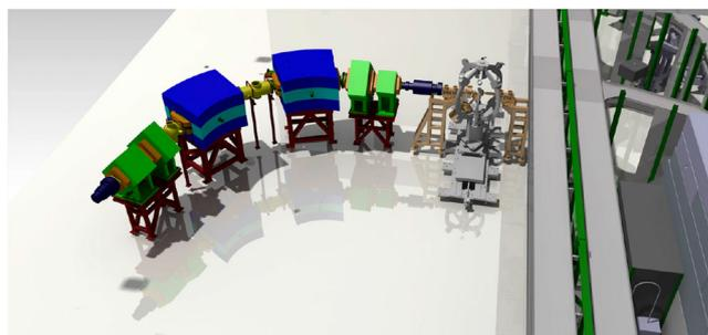
**Fig. 15.** 3D drawing of the possible integration of a zero-degree spectrometer after the MINIBALL array for the identification of the ejectiles in transfer reactions of high energy.
