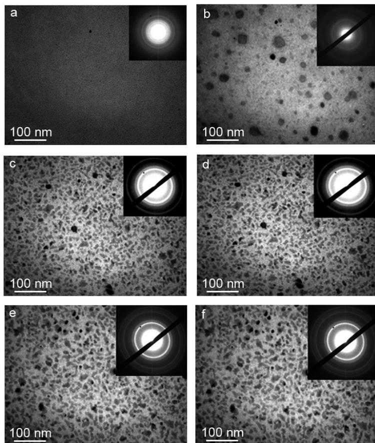
**Fig. 3.** The structure of ultrathin films of CoNi alloy. (a) as-deposited film; (b)–(f) after annealing to 700 K. The effective thickness of the films: (a) 20 nm ( $c_{\text{Co}} = 20\%$ ); (b) 9 nm ( $c_{\text{Co}} = 80\%$ ); (c) 9 nm ( $c_{\text{Co}} = 10\%$ ); (d) 10 nm ( $c_{\text{Co}} = 30\%$ ); (e) 15 nm ( $c_{\text{Co}} = 70\%$ ); (f) 20 nm ( $c_{\text{Co}} = 50\%$ ).
